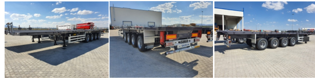
MECHANICAL SUSPENSION 4 X 14 T AXLE TIRES 12 R 22,5 - 16+1 PCS
